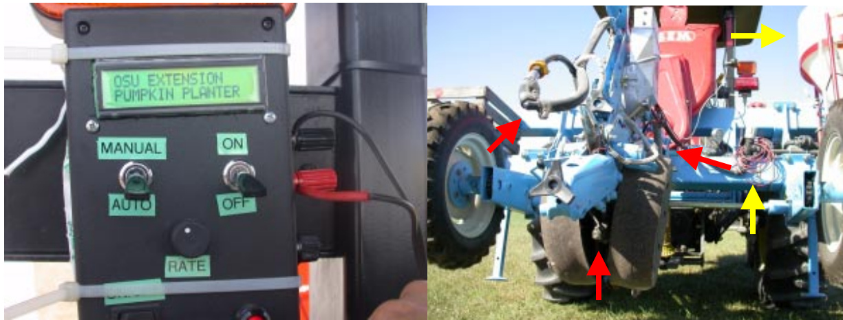
Figure 1. A picture of both the cab mounted controller box on the left and rear shot of planter and most of injector on the right. The tank and electric pump are visible on the right hand side of the planter (yellow arrows). Most of the plumbing, solenoid, and nozzle can also be seen (red arrows).
